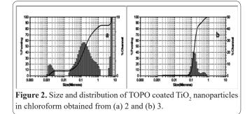
dary particle sizes of 174 nm, 165 nm and 312 nm with almost uniform distribution.
