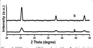
Figure 1. XRD paterns of  $TiO_2$  synthesized from 2 calcined at (a) 400°C and (b) 600°C.
