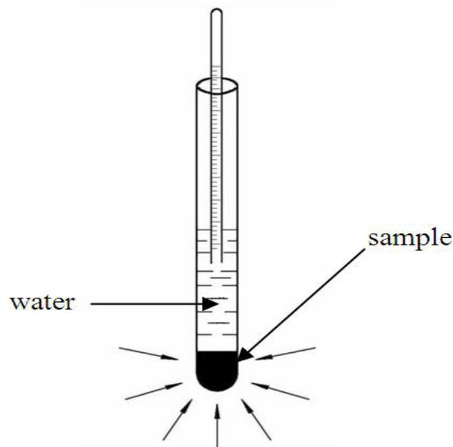
Figure 1. schematic diagram of liquid dilatometer.
